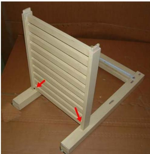
Insert shelf (D) into slots in leg assembly (B), ensuring the screw holes are on the underside. Fix shelf using 2 large screws shown by arrows.
